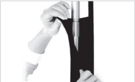
3. Attach the fabric with velcro to the frame in a wrapping motion.
