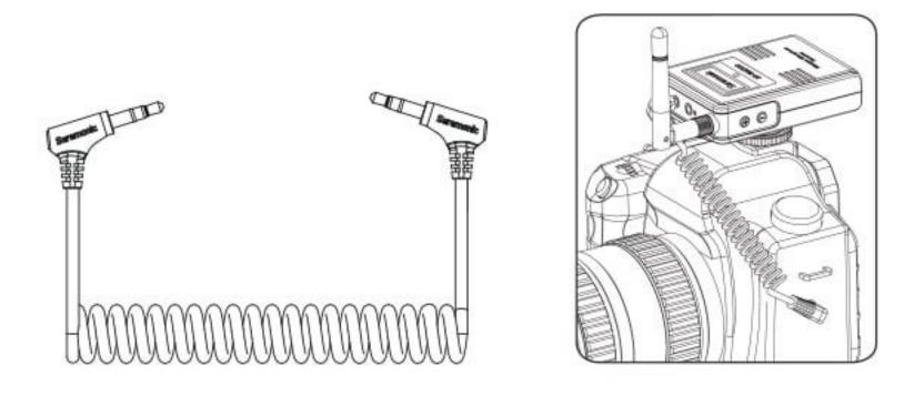
When connecting to a smartphone, tablet or computer, please use the 3.5mm TRS to TRRS (CTIA standard) output cable. Plug the 90 degree right angle TRS into the line output jack of the receiver and plug the straight TRRS end into the 3.5mm headphone jack of a smartphone, tablet, or computer.
