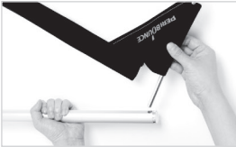
3. Place the rod at each connecting point and tilt the angle of entry of the rods at (approx. 15degree angle) to the frame body then insert to complete the full "U" Frame
