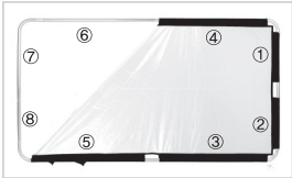
4. Attach the fabric one side at a time then proceed to other side.
